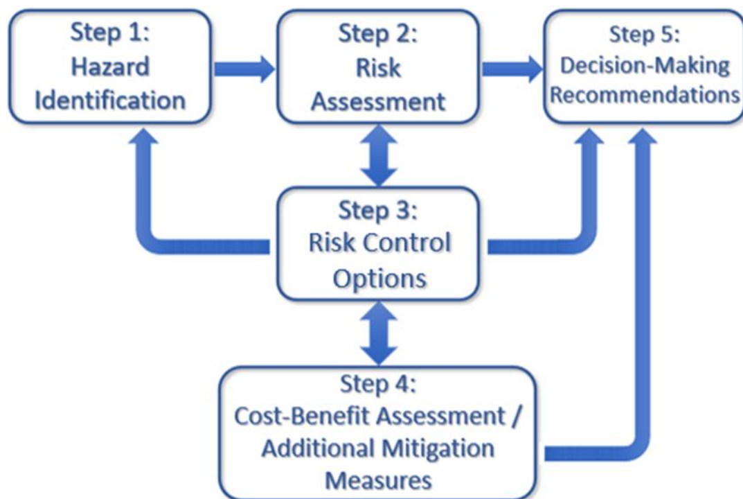
Figure 15.1.1 Flow chart of the FSA methodology
